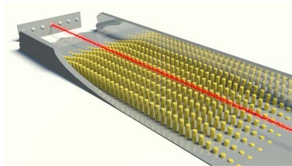
One of the attractive features of this concept is the possibility to stream more than one electron beam through the photonic crystal. This has two major advantages, (i) it allows to scale the output power of the device and (ii) it relaxes the requirements on the electron generation (electron gun) and electron beam transport through these devices.
